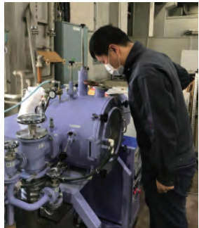
Adding element Sr and Ca into melted magnesium alloy by using casting equipment
